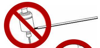
**Never hold the stop arm by hand.** On reversal, full power of the machine is transmitted through the stop arm and the operator could be seriously injured.
