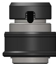
**Hard Start:** Use this position for drilling. Push up against the QC spindle and it should not compress. May also be used for tapping. Hard start can help make the tapping depth more consistent. **Self Feed for tapping in this position: Size 50, 3 to 4mm.**
